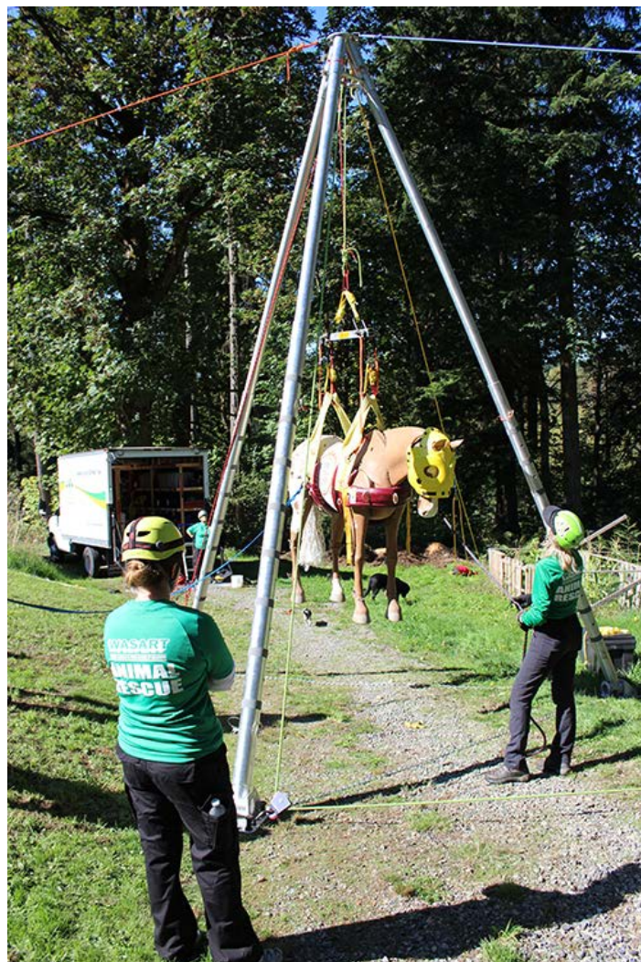
The tripod is used to hoist larger animals straight up. The tripod and sling used on the horse were both designed by Dr. Becker, a veterinarian and engineer.
